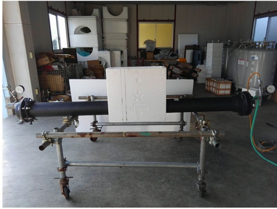
Figure 1. Single-ice-plug freezing: B = 480, 520 and 560 mm.
